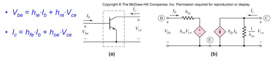
where the subscripts are: *i* for input, *r* for reverse, *f* for forward, *o* for output, and *e* for common emitter.
