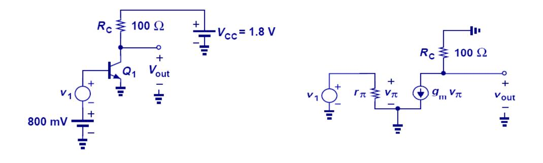
The circuit of Fig. 4.24(a) is modified as shown in Fig. 4.25, where resistor  $R_C$  converts the collector current to a voltage. (a) Verify that the transistor operates in the active mode. (b) Determine the output signal level if the microphone produces a 1-mV signal.
