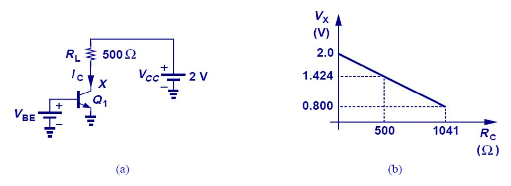
Figure 4.14. (a) Simple stage with biasing, (b) variation of collector voltage as a function of collector resistance.
