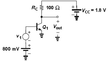
Considering the previous Example, suppose we raise  $R_C$  to 200 $\Omega$  and  $V_{CC}$  to 3.6 V. Verify that the device operates in the active mode and compute the voltage gain.
