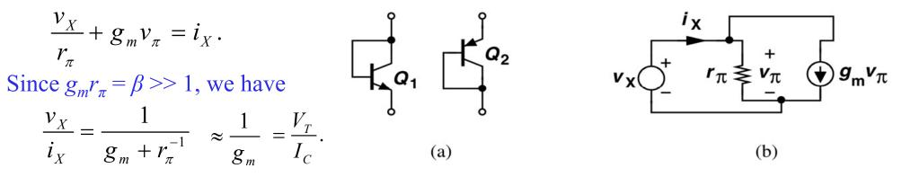
Interestingly, with a bias current of  $I_C$ , the device exhibits an impedance similar to that of a diode carrying the same bias current. We call this structure a "*diode-connected transistor*." The same results apply to the *pnp* configuration in Fig. 4.44(a).
