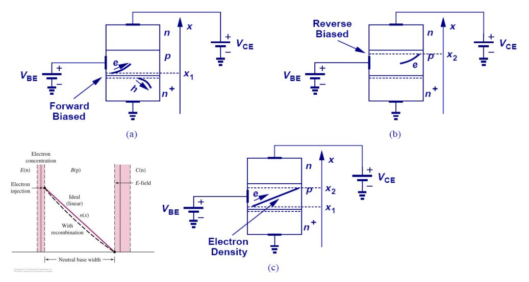
The electron density gradient in the base provides the diffusion of electrons.
