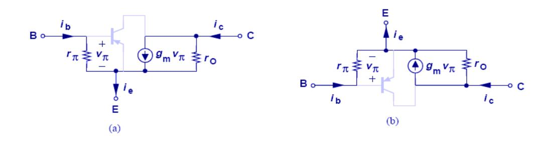
If the collector and base of a bipolar transistor are tied together, a two-terminal device results. Determine the small-signal impedance of the devices shown in Fig. 4.44(a). Assume  $V_A = \infty$ .
