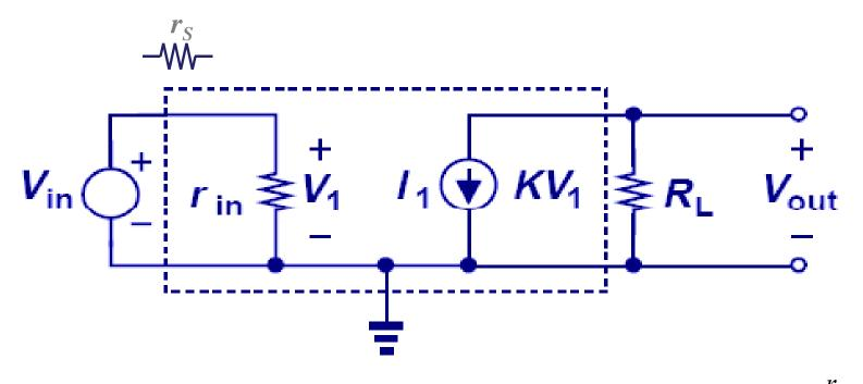
$V_{in}$  usually exists a source resistance,  $r_S$ , which will degrade the gain by a factor  $\frac{r_{in}}{r_{in} + r_S}$
