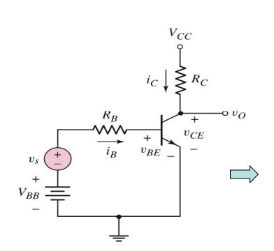
$V_o = -(g_m V_\pi) R_C, (\because V_\pi = \left(\frac{r_\pi}{r_\pi + R_R}\right) \cdot V_s)$  $\Rightarrow A_{\nu} = -(g_{m}R_{C})\cdot\left(\frac{r_{\pi}}{r_{-}+R_{n}}\right)$  $I_c$  $\bigcirc$  $R_{R}$ B  $\circ V_o$ +  $g_m V_{be} =$  $V_{\pi} = V_{be} \stackrel{i}{\leqslant} r_{\pi}$  $\leq R_C$  $V_{\rm s}$  $g_m V_\pi$ E Copyright © The McGraw-Hill Companies, Inc on required for reproduction or display
