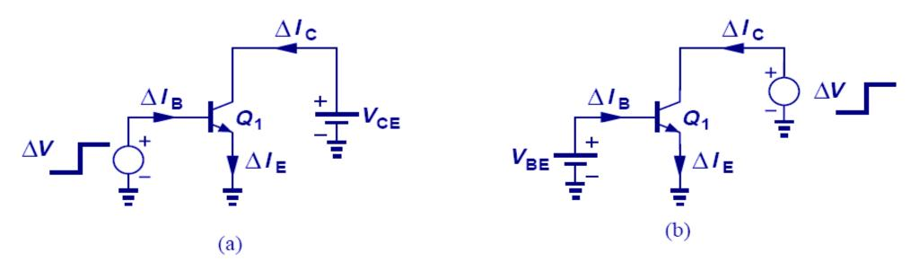
Small changes in (a) base-emitter ( $V_{BE}$ ) and (b) collector-emitter ( $V_{CE}$ ) voltage.
