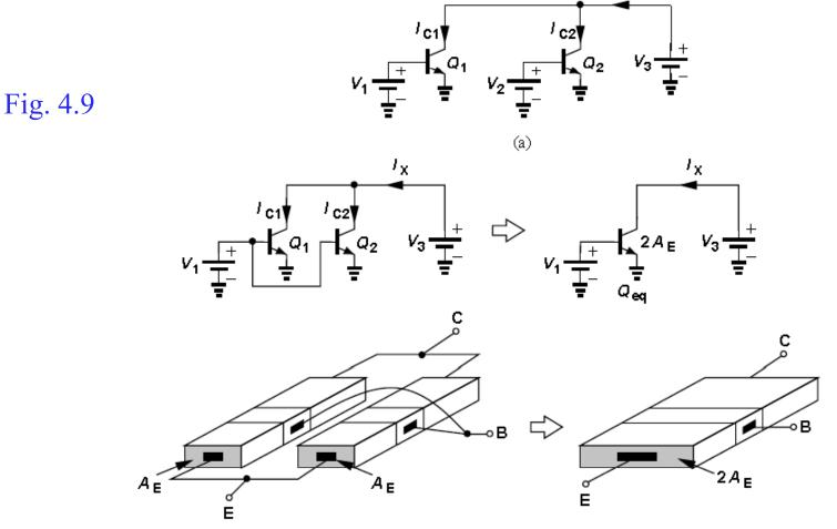
Determine the current  $I_X$  in Fig. 4.9(a) if  $Q_1$  and  $Q_2$  are identical and operate in the active mode and  $V_1 = V_2$ .
