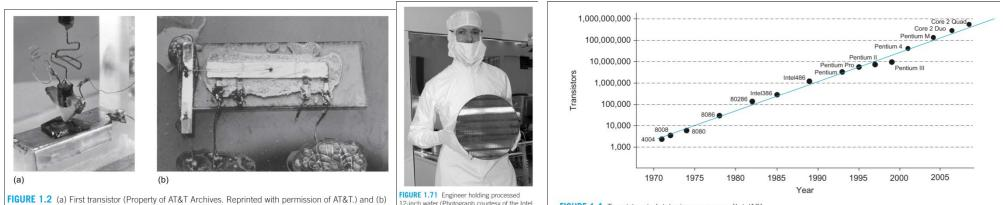
FIGURE 1.2 (a) First transistor (Property of AT&T Archives. Reprinted with permission of AT&T.) and (b) first integrated circuit (Courtesy of Texas Instruments.)
