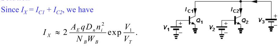
This result can also be viewed as the collector current of a single transistor having an emitter area of  $2A_E$ . In fact, redrawing the circuit as shown in Fig. 4.9(b) and noting that  $Q_1$  and  $Q_2$  experience identical voltages at their respective terminals, we say the two transistors are "in parallel," operating as a single transistor with twice the emitter area of each.
