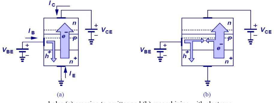
holes (a) crossing to emitter and (b) recombining with electrons.
