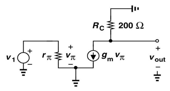
Fig. 4.26 Small-signal equivalent circuit of the stage shown in Fig. 4.25.
