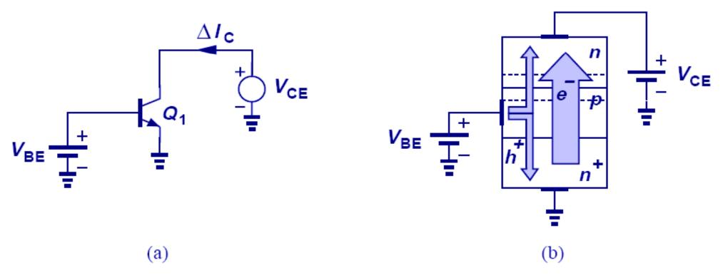
A bipolar transistor is biased with  $V_{BE} = 750 \text{ mV}$  and has a nominal  $\beta$  of 100. How much B-C forward bias can the device tolerate if  $\beta$  must not degrade by more than 10%? For simplicity, assume base-collector and base-emitter junctions have identical structures and doping levels.
