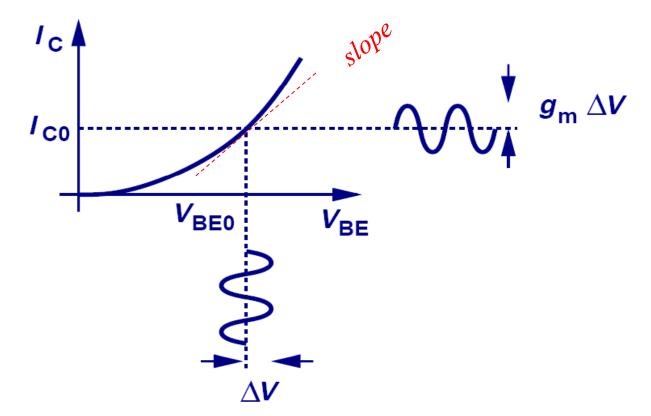
The *bias* (or called *quiescent*, *operating*, or just Q) point is  $(V_{BE0}, I_{C0})$ . Around the point, a small signal change,  $\Delta V$ , generate a larger signal,  $g_m \Delta V$
